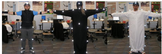
Figure 2. MoCap suits with markers: Western (L), Emirati Women (M), Emirati Men (R). Notice the CyberGlove on the left hand in L
